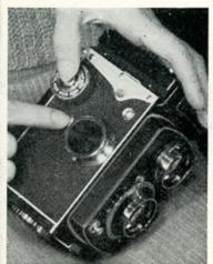
While pressing the Film Winding Knob Release, pull down the Film Counting Reverse Button so that the Film Counting Dial shows "S".
