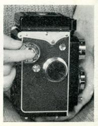
again press the Film Winding Knob Release Button and turn the Film Winding Knob so that the Film Counting Dial shows the next number. The Film Winding Knob will lock automatically.
