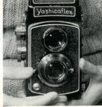
Push down the Shutter Cocking Lever. Be sure not to change Shutter Speed after the shutter is cocked.
