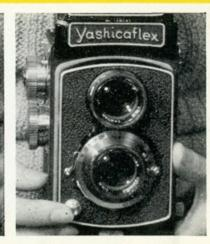
Catch the object on the Ground Glass Screen or the Sports Finder. Now gently release the Shutter by pressing the release button.
