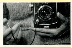
A Time exposure longer than 1/10 sec. may be obtained by using the cable release. Set the shutter at B (bulb) position.
