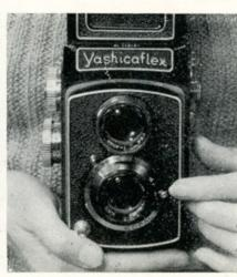
The Lens Aperture Opening is controlled by the Lens Aperture Control Lever by using an exposure meter or exposure
