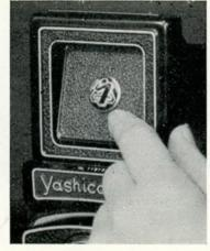
The Magnifying Glass is for more accurate focusing. Erect the Magnifying Glass by pressing the top of the Focusing Hood.
