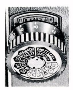
By use of this Depth-of-Field scale, your Yashica will also become a fixed-focus camera. In this case set the distance scale to 15 feet (5m) and the lens aperture to f:8. You will notice on the Depth-of-Field that anything from about 10 feet (3.5m) to 23 feet (9m) will be in focus.
